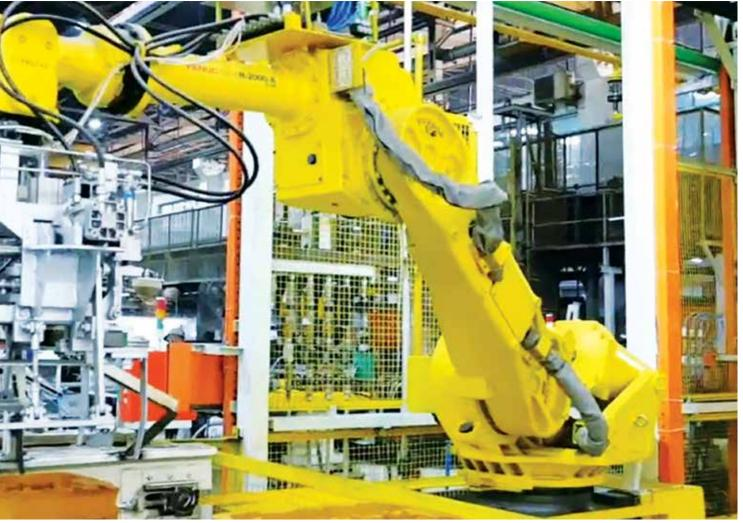
Automatic GDC production line with robots for 4W Clyinder head
